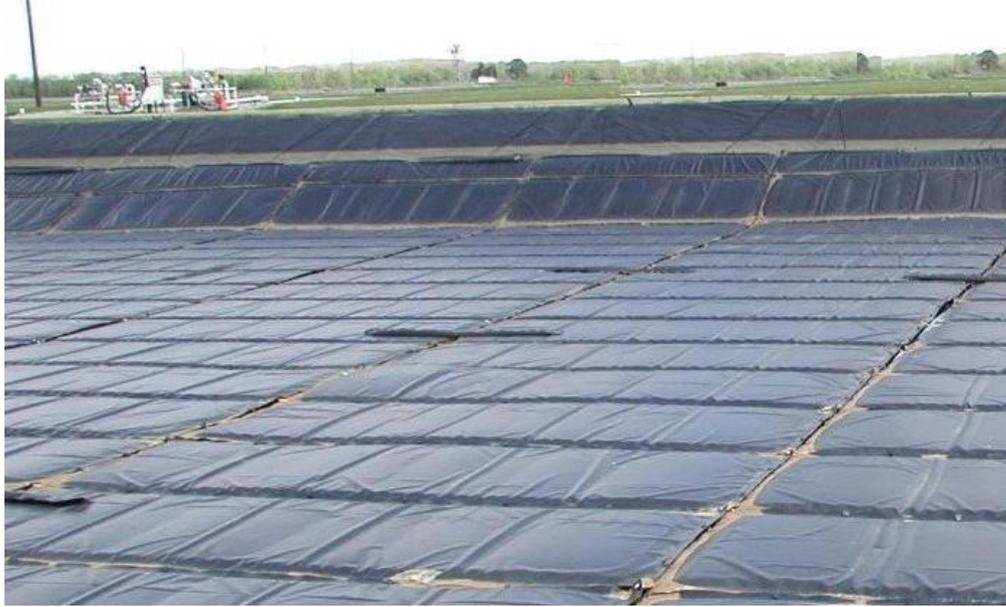
During winter months it can be expensive and difficult to keep water from freezing for use in hydraulic fracturing procedures. Heating costs can be dramatically decreased by the use of insulating floating covers to help prevent heat loss of the open body of water. Whether your application is a lined earthen pit or an aboveground steel water tank, Contain Enviro can custom suit your requirements.
